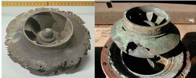
Two badly worn centrifugal pump impellers
